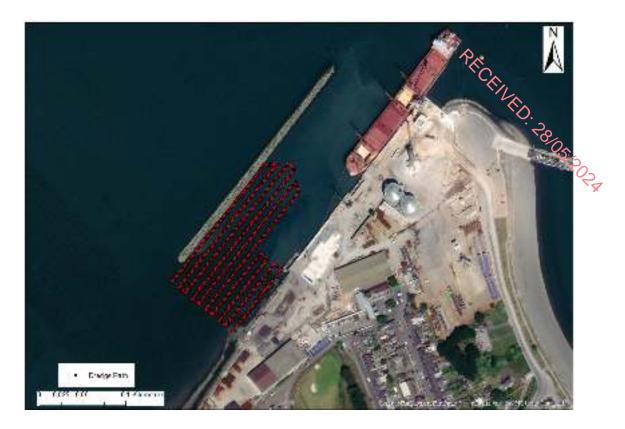
Figure 12.27 Dredge path used in the model for suspended sediments.
